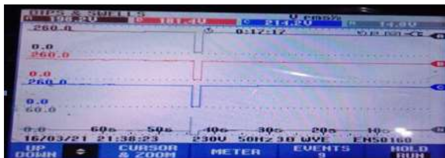
Figure 9: Result on Power Quality Analyzer on sag condition
