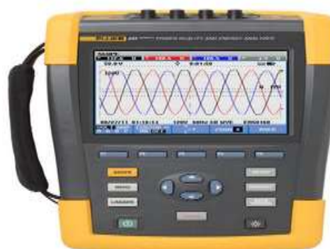
Figure 4: Variable Power Supply Figure 5: Power Quality and Energy Analyzer Fluke 435
