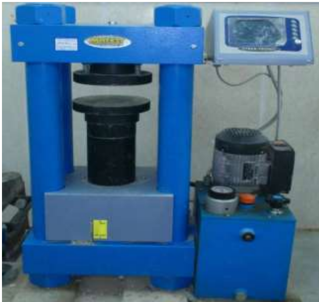
Fig 3.5 Compressive strength test machine
