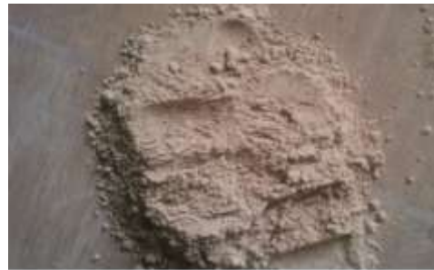
3.2 Fig pulverized waste ceramic tiles
