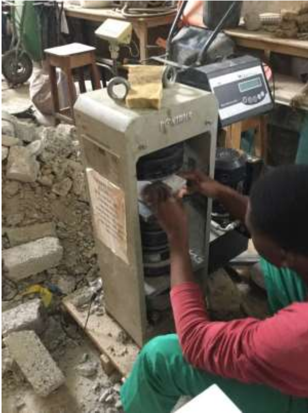
Fig : compressive strength test on concrete samples
