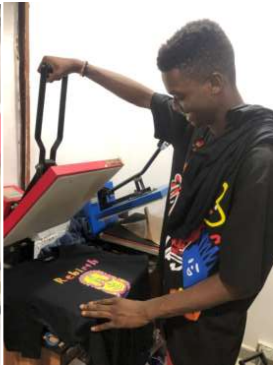
Plate 7: Using the heat transfer machine to transfer the design on T-shirt
