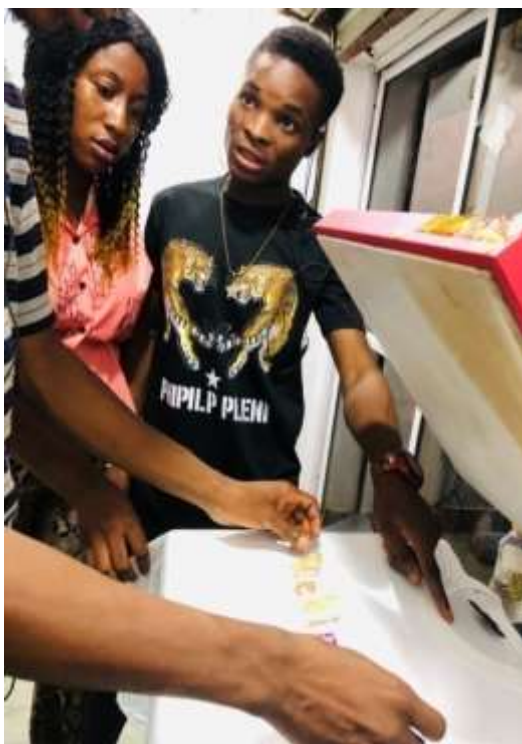
Plate 6: Placing the T-shirt for the heat transfer Photograph by George G. Odey (2021)
