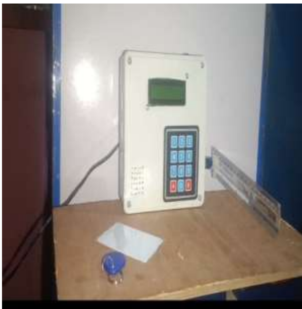
Figure 11 Picture of the Constructed Toll Tax System
