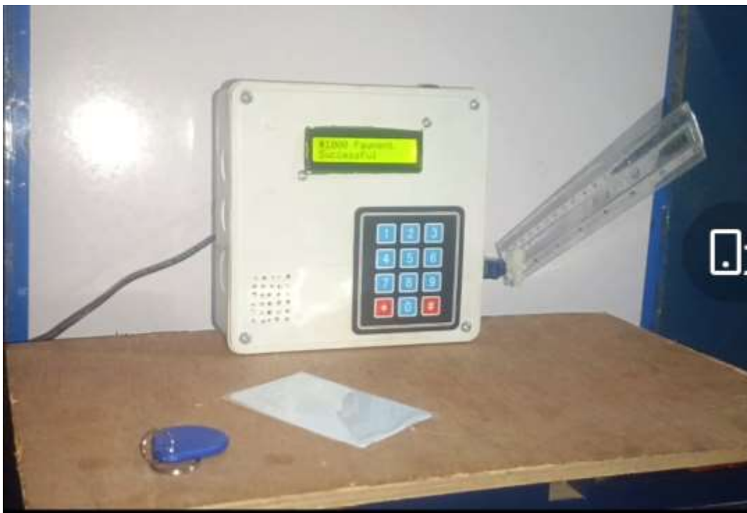
Figure 15 the Servo is Witched on to Drive the Motor to Give Access
