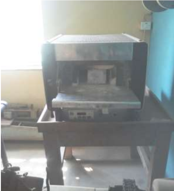
Figure 3 Heating of the samples in a furnace
