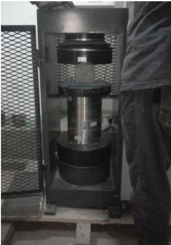
Figure 4 Compression Test of Concrete Cubes
