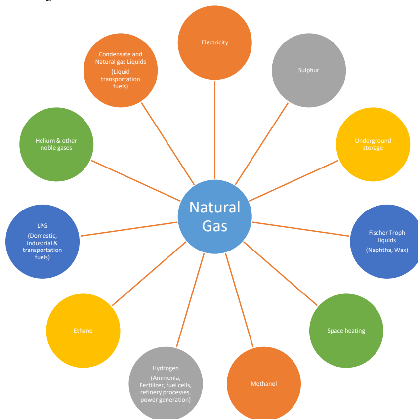
Figure 14:A global framework of the expected AKK based natural gas process extraction, utilization and conversion routes. Source:(Nwaoha, 2014)
