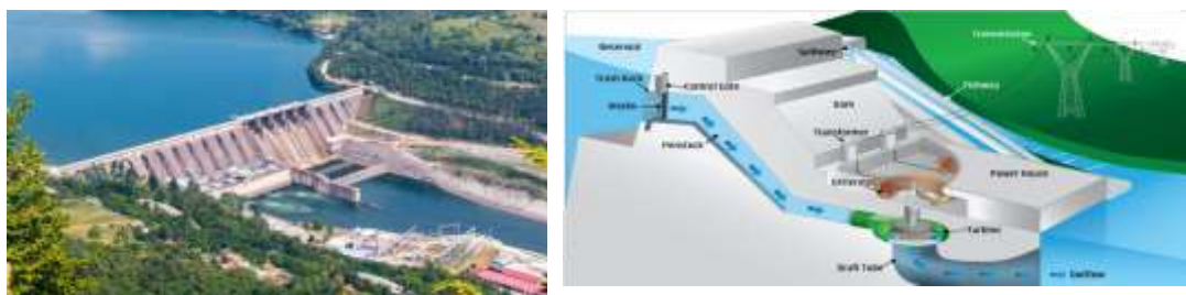
Figure 1: Illustration of the concept of a hydroelectricity dam and the power generation scheme
