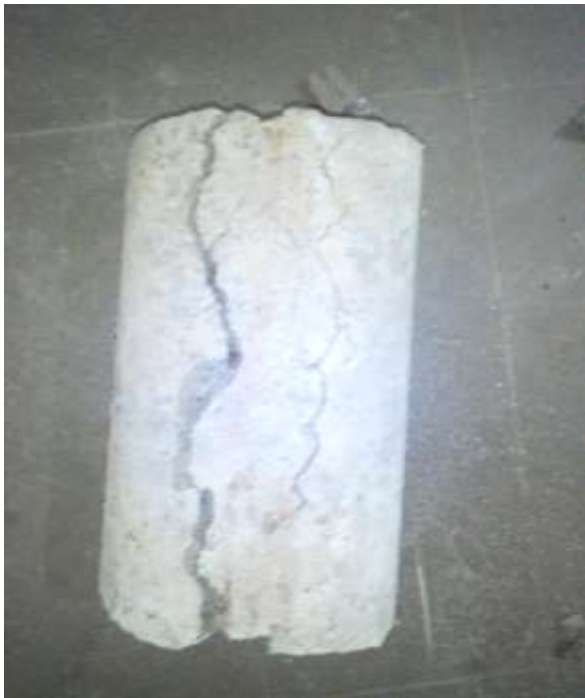
Figure 3: Split Tensile Cylinder Samples after Failure
