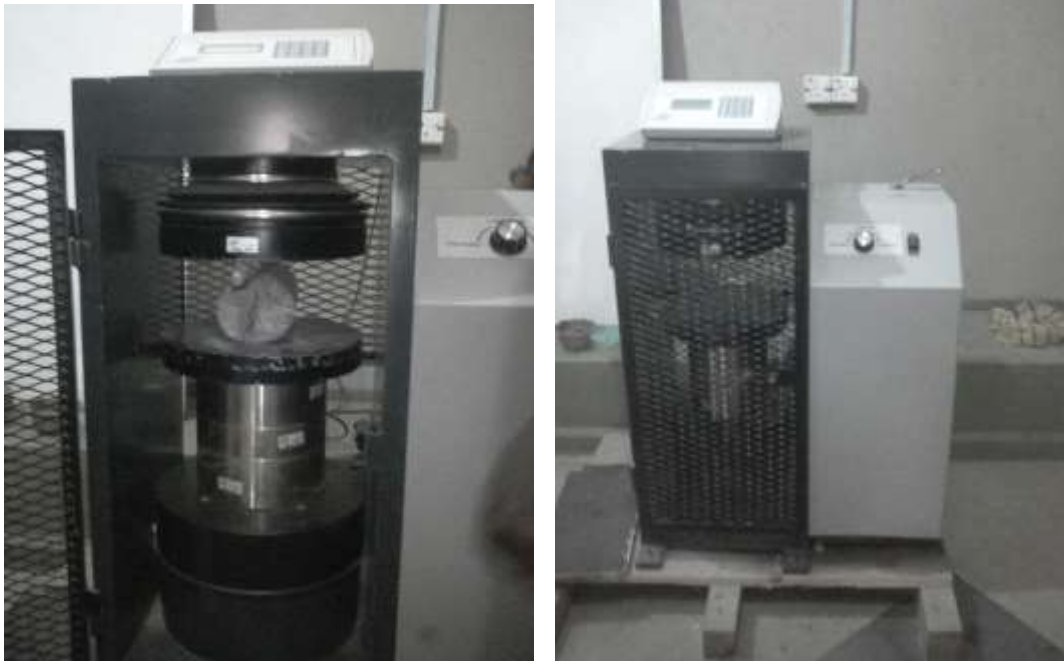
Figure 2: Compression Test Machine used in the experiment Cylinder Sample
