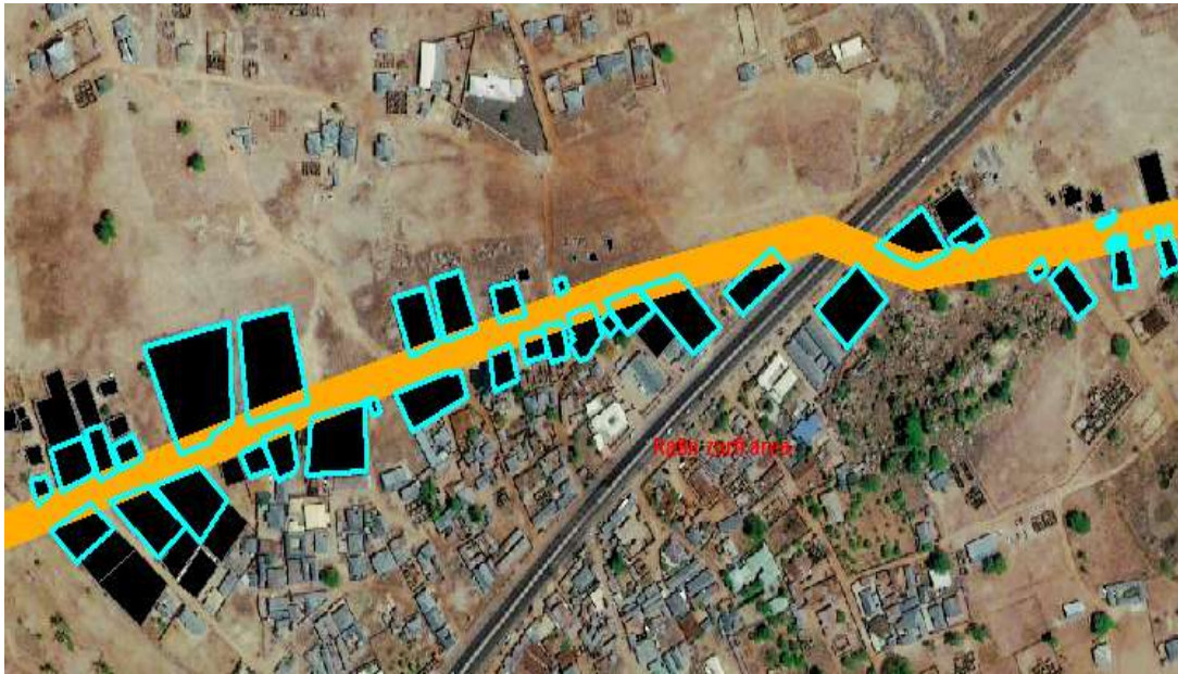
Figure 1: Spatial query showing properties that encroached pipeline at Rafin zurfi area
