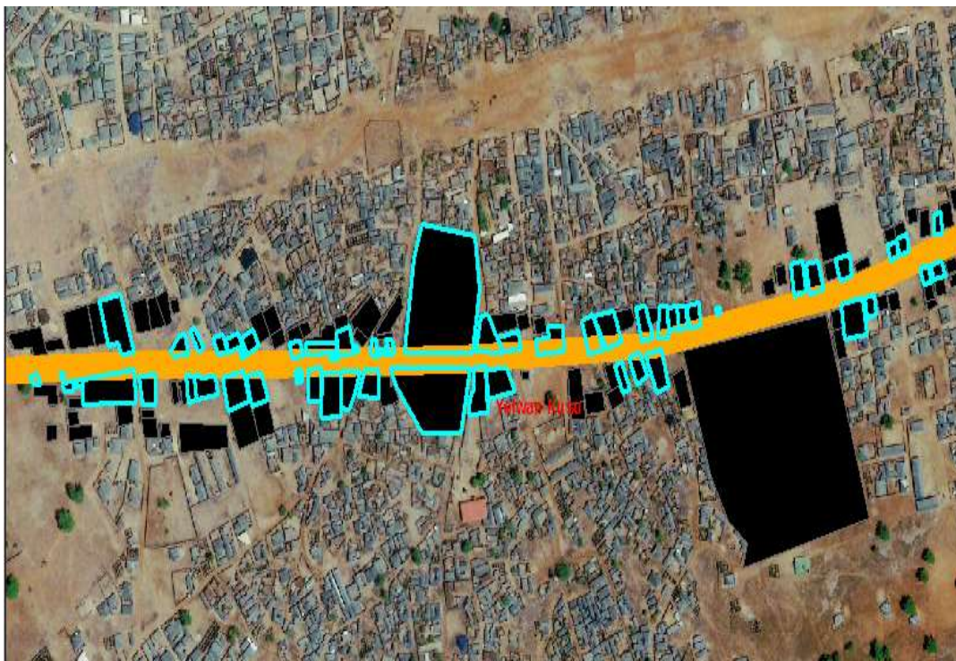
Figure 2: Spatial query showing properties that encroached pipeline at kusu area of yelwa
