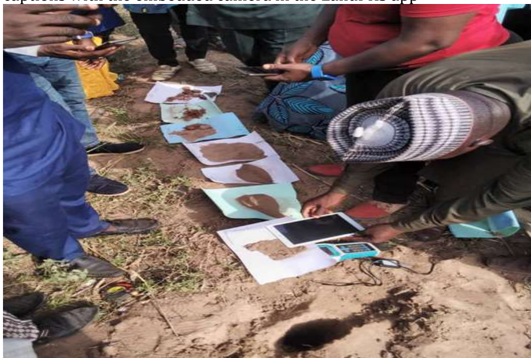
Fig3: Photography showing Testing for soil texture, soil color by photo captions with the embedded camera in the LandPKS app
