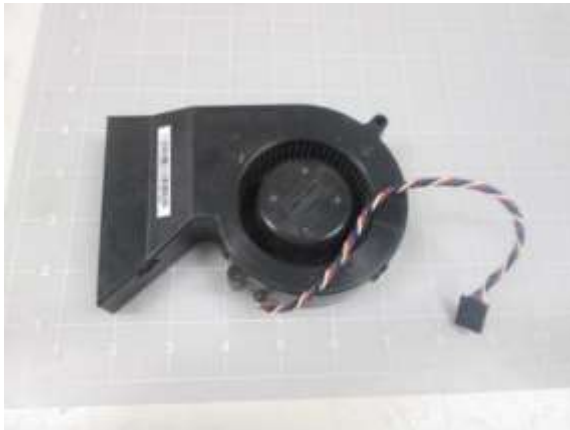
Figure 7: Suction Fan 12 VDC 2.65A
