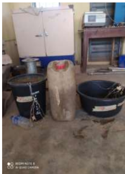
Plate 3.0: Samples embedded in Fresh water, Seawater and Sea sand.
