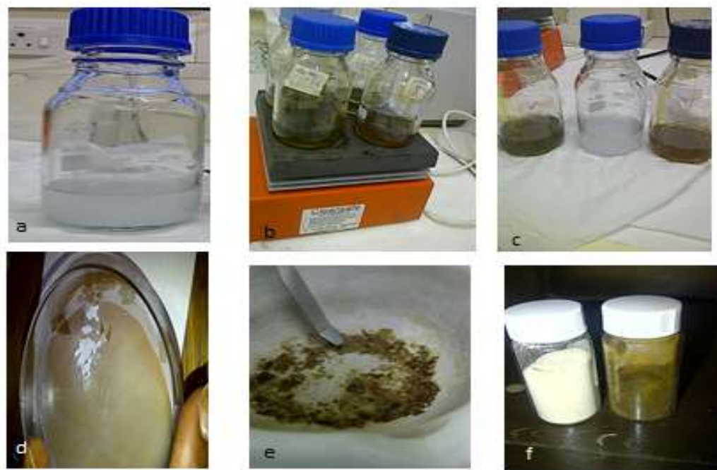
Figure 1: The step-wise synthesis of starch silver nanoparticles where a, is the starch- \text{AgNO}_3 -glucose complex, b-e the steps and f (brown) the end product.
