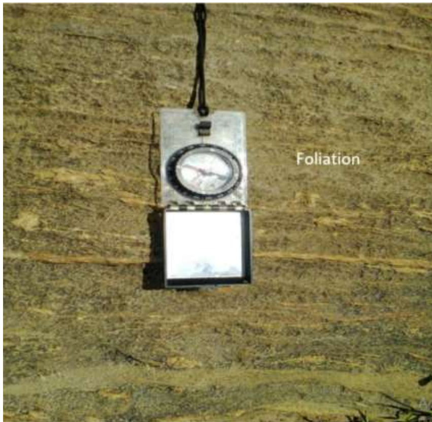
Plate. 3.10: Foliation on granite-gneiss at Marke ( 8^{\circ}50'08''N , 7^{\circ}59'50''E ). The compass is oriented in the regional trend of the area (NNW-SSE).
