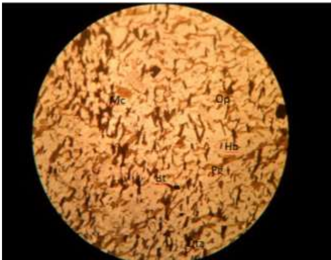
Plate 3.6a: Photomicrograph of banded-gneiss under plane polarized light (Magnification X40)
