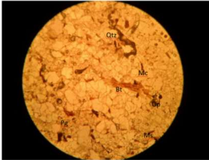
Plate 3.4a: Photomicrograph of foliation in granite-gneiss under plane polarized light (Magnification X40)
