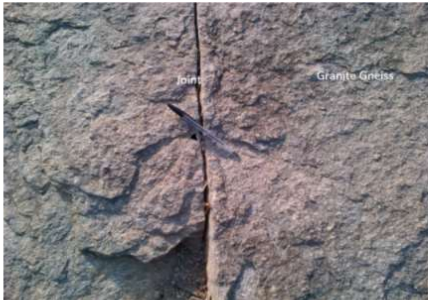
Plate 3.11: Joint on granite gneiss ( 8^{\circ}50'10'' N, 7^{\circ}54'57'' E)
