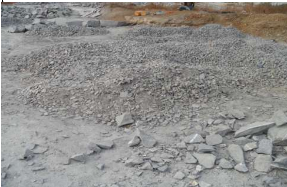
Plate 4.1: Quarried granite gneiss for building purposes (8 0 47'21''N,7 0 59'58''E)
