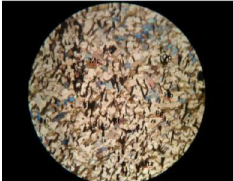
Plate 3.6b: Photomicrograph of banded-gneiss under cross polarized light (Magnification X40)
