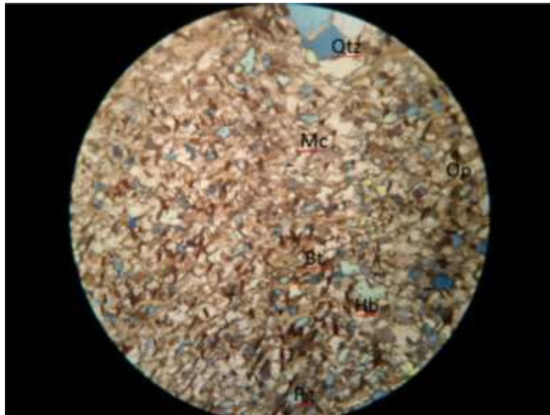
Plate 3.7b: Photomicrograph of banded-gneiss under Cross Polarized Light (Magnification X40)
