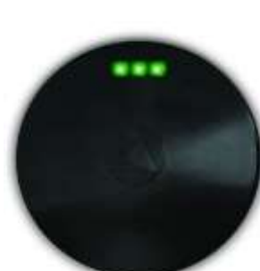
Fig.7: Three green LEDs indicates the device successfully register itself with our servers
