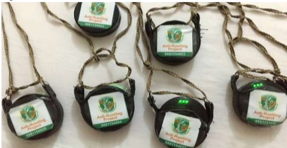
Figure 3: Fabricated Tracking chips with jackets
