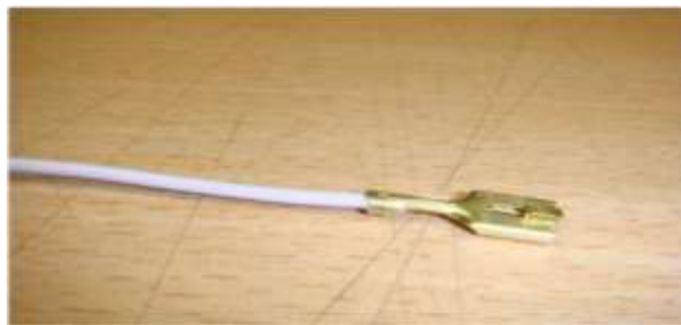
Figure 4(b): Terminal Lock Bend condition
