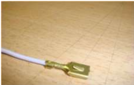
Figure 4(a): Terminal locks correct
