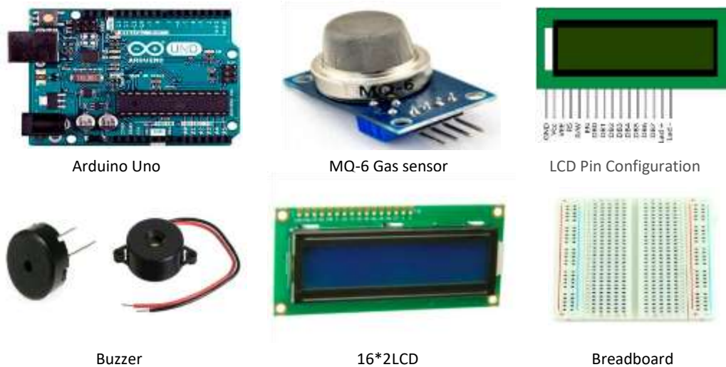
Figure 2. Some important components that are needed to design the gas leakage detection and alert system.
