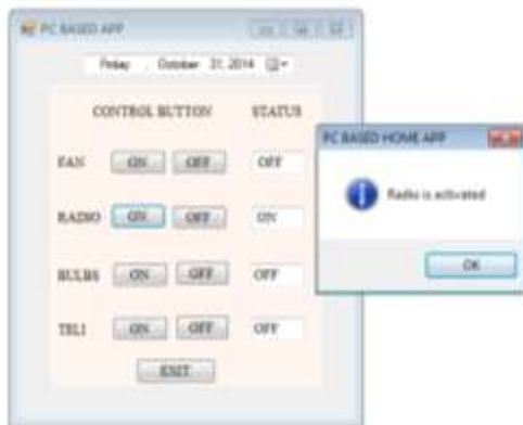
Figure 9: Message displayed When RADIO is switched ON
