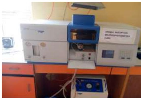
Figure 3.5: AA320N model of Atomic Absorption spectrophotometer
