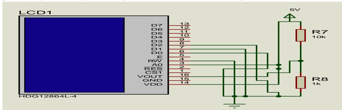
Fig. 4: LCD circuitry with Constant Dividers
