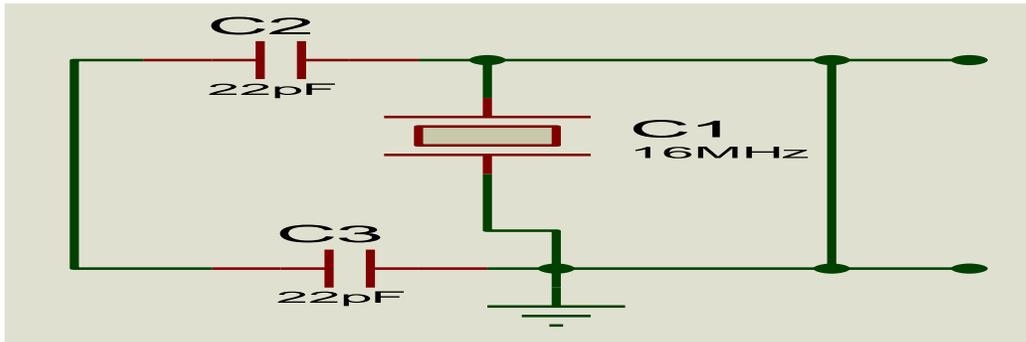
Figure 5: Oscillatory Circuitry for Microcontroller.
