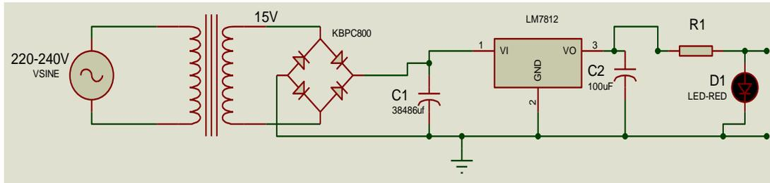
Fig.2: 12V Power Supply Circuit
