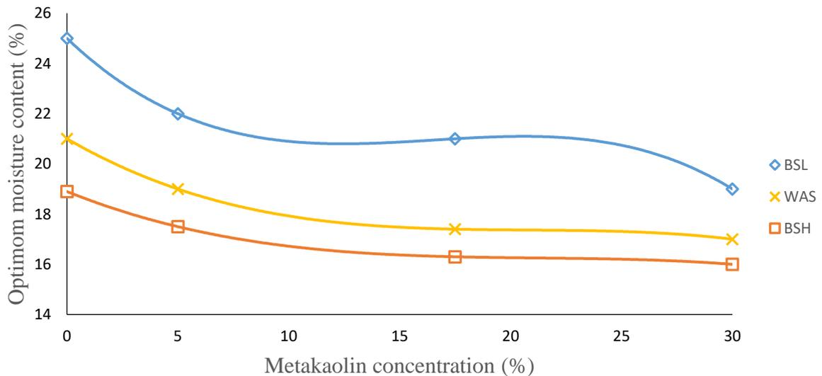
**Figure 6:** Variation of Optimum Moisture Content of Non- Lateritic Soil with Metakaolin
