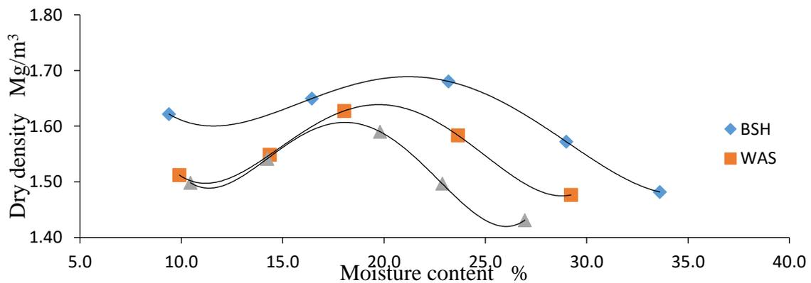
Figure 3: Moisture - Density Relationship of the Non-Lateritic Soil (NLS)
