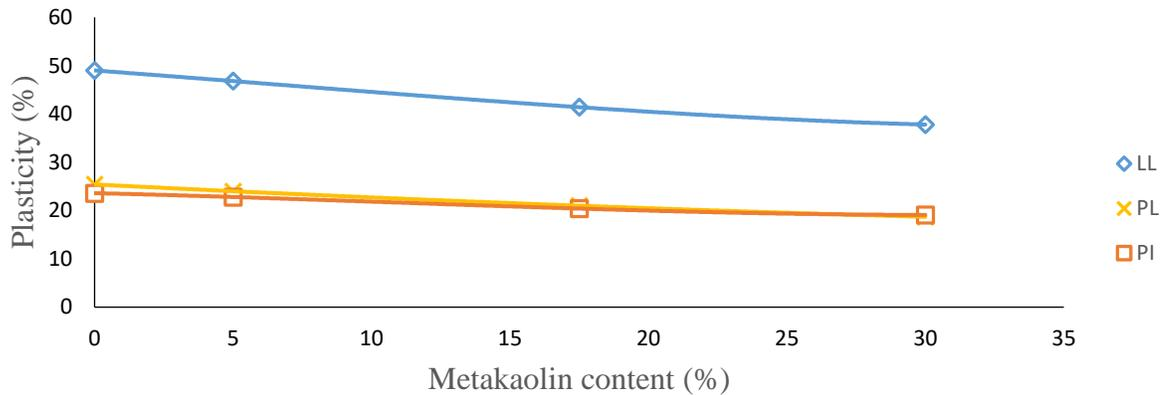
Figure 2: Variation of Atterberg limits of NLS treated with MK content
