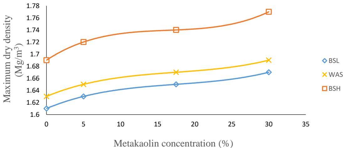
**Figure 5:** Variation of Maximum Dry Density of Non-Lateritic Soil with Metakaolin
