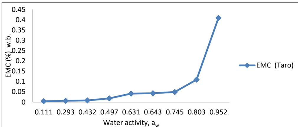
Figure 4: Adsorption isotherm of taro at 60 °C
